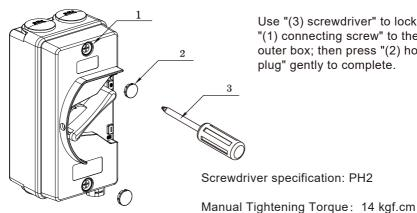
Use "(3) screwdriver" to lock "(1) connecting screw" to the outer box; then press "(2) hole plug" gently to complete.
